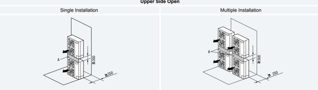
Close the part A not to allow the outlet air bypassed. Install to avoid the drain water from upper unit falling on the lower unit.
