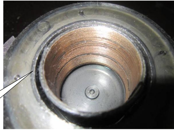
The scroll plate is worn.
