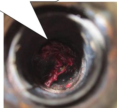
The filter is blocked by impurity, the suction of the compressor will be abnormal
