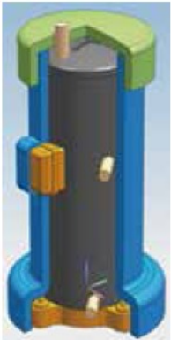
Integrated type sound absorber
