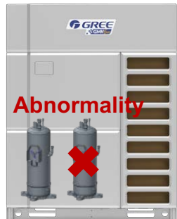
Compressor emergency operation
